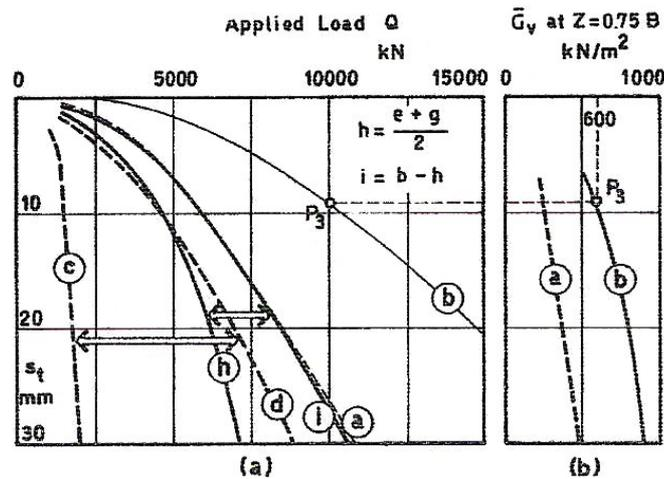
FIG. 8. APPLIED LOAD AGAINST PILE TIP SETTLEMENT DIAGRAM
