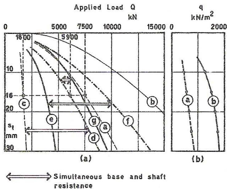
**FIG. 6. APPLIED LOAD AGAINST PILE TIP SETTLEMENT DIAGRAM**
