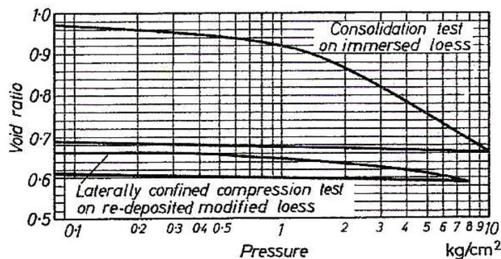
**Fig. 5 Results of consolidation test on a saturated sample of immersed loess and of a laterally confined compression test on a re-deposited modified loess**
