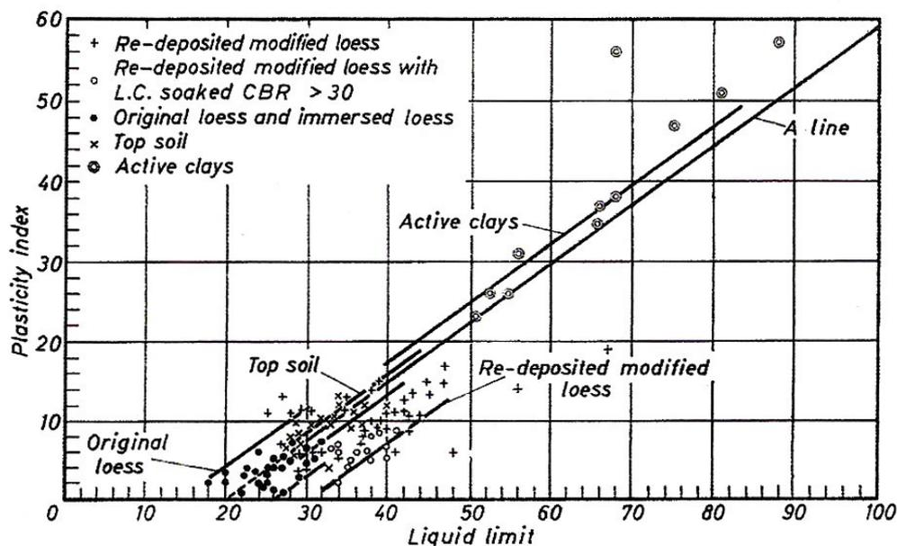
**Fig. 1 Plasticity chart showing the position of original and modified loess, top soil and active clays**
