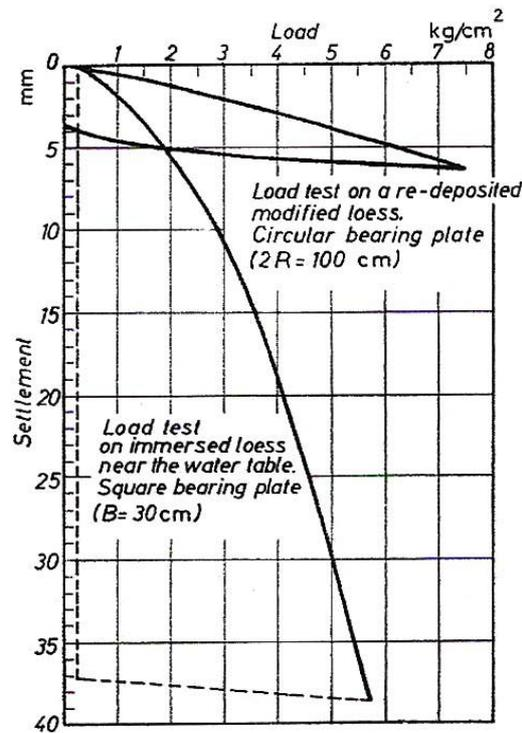
**Fig. 4 Results of load tests performed on the upper layers, near the water table, of an immersed loess and on a re-deposited modified loess**
