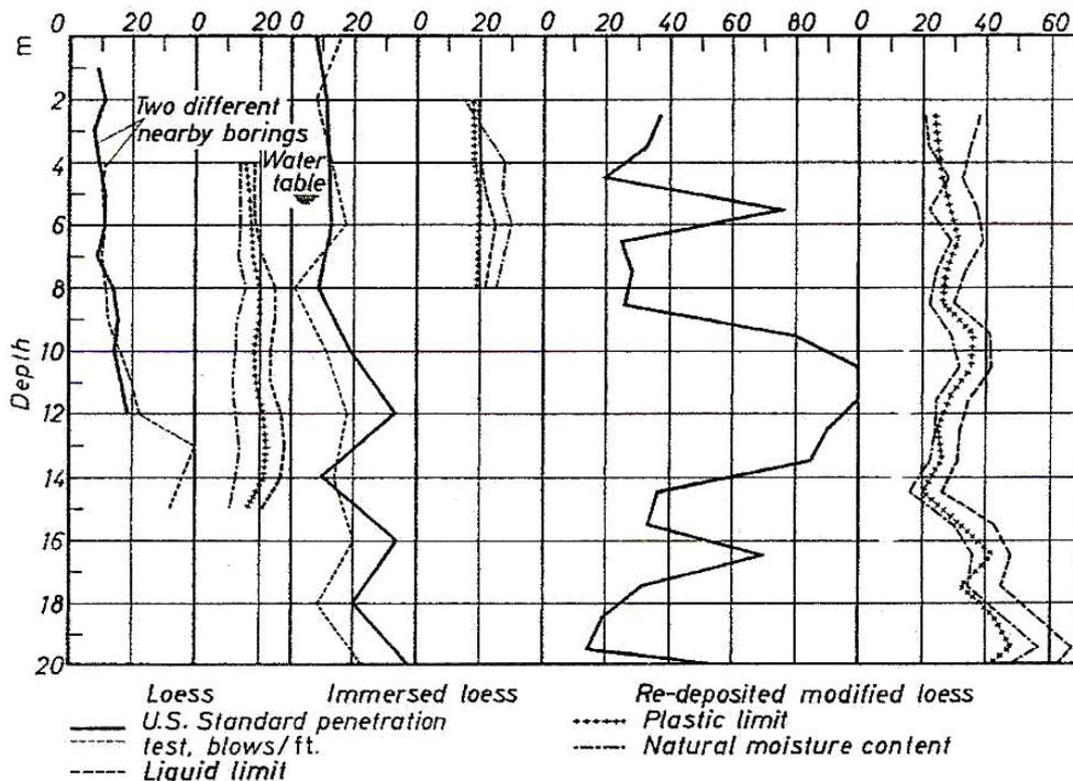
**Fig. 3. Results of U.S. standard penetration tests, liquid limit, plastic limit and natural moisture content, performed on deposits of original, immersed and re-deposited modified loess**
